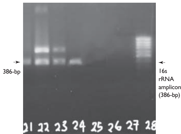
Figure 1. Gel electrophoresis picture of 16s rRNA gene PCR for Legionella spp. Lanes 21-24: water samples positive for Legionellae ; lanes 25-27: negative controls; lane 28: 100-bp marker. The specific 16s rRNA amplicon appears as a 386-bp band. The second (649-bp) band in lanes 22 and 23 is the product of amplification of a virulence gene in Legionella pneumophila (not described in this study).
