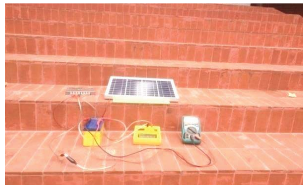
Fig. 8. Solar panel, DC Ammeter, Voltmeter, Battery, & Charge Controller used for data collection (without shading).
