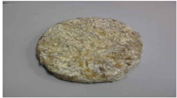
Figure 3 The constructed sound absorber sample from the paddy straw fibers.
