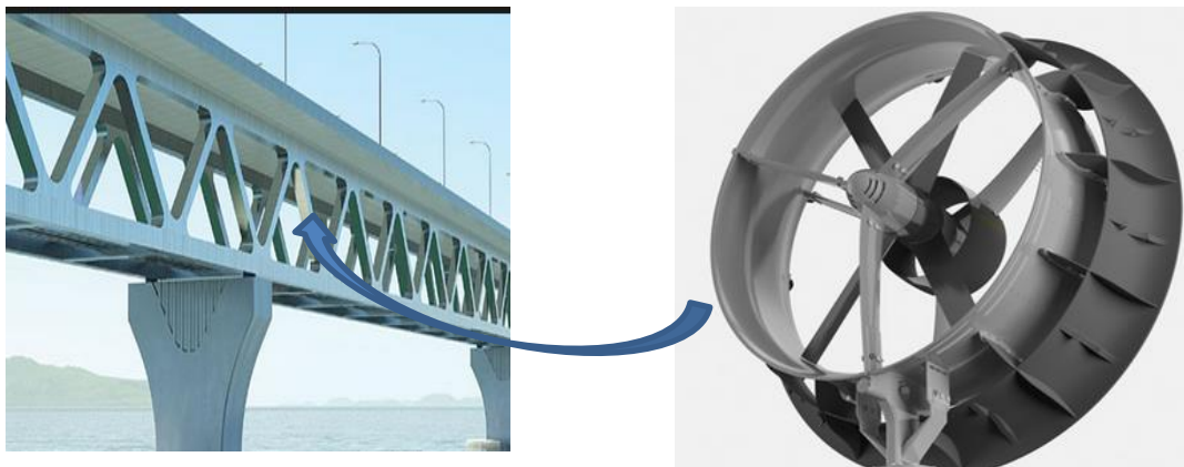
Figure 10 Wind turbine installed place in the bridge
